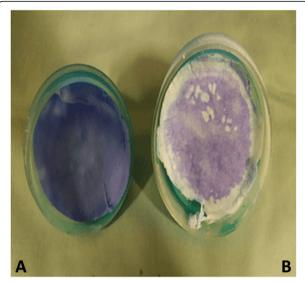
**Fig. 1** Illustration of the dye leak test. **a** 1.5  $\mu$ m filter paper with dye leaking around the edges. **b** 1.5  $\mu$ m filter paper where all the dye has passed through the filter material without leaking around the edges
