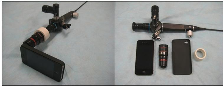
**Figure 1** Fiberoptic bronchoscope with iPhone, lens, and rubber attachment.
