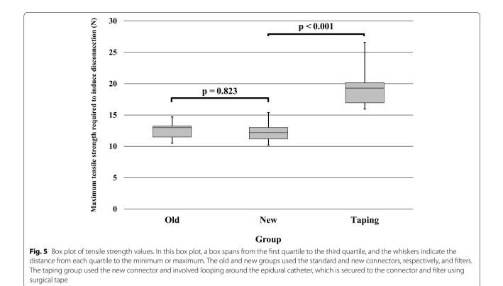
analysis of the new and taping groups indicated that disconnection occurred less frequently in the taping group. In this laboratory study, there was no significant difference in the tensile strength required for disconnection between the new and old groups, but there was a significant difference between the new and taping groups.
