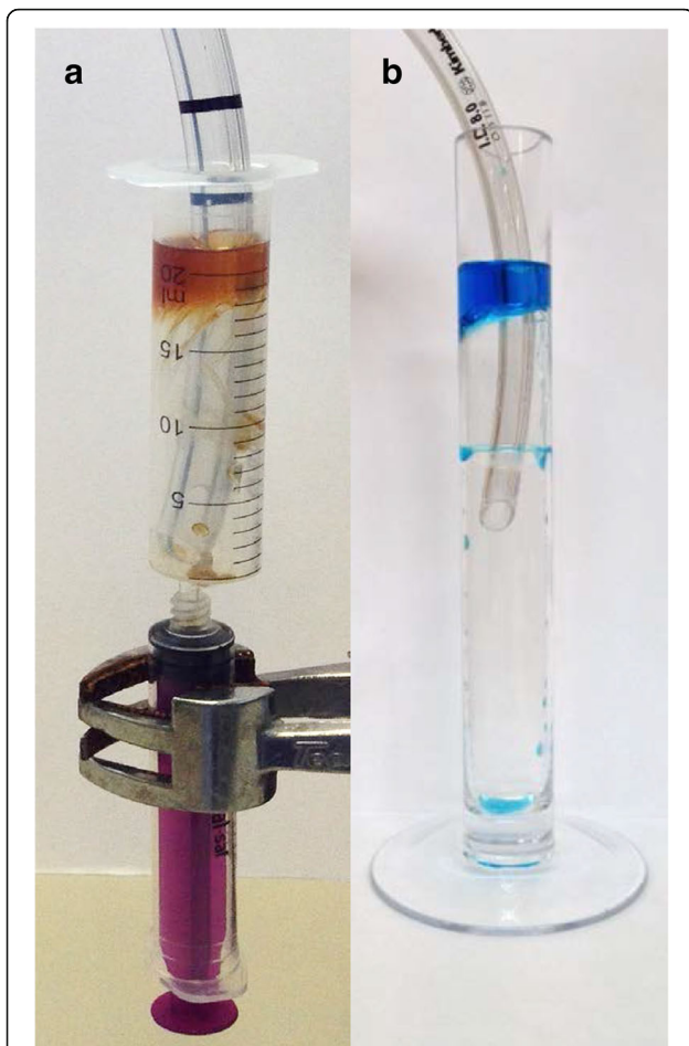
Fig. 2 a The in vitro trachea model used in the aspiration of microbial fluid study. The 20 ml syringe was connected to the 10 ml enteral syringe via the tip. The endotracheal tube was placed in the 20 ml syringe. Fluid leaking past the cuff was collected aseptically in the enteral syringe. b the in vitro trachea model used in the range of tracheas study. The endotracheal tube was placed inside the rigid glass 'trachea' and the fluid leaked past the cuff was collected inside the model
