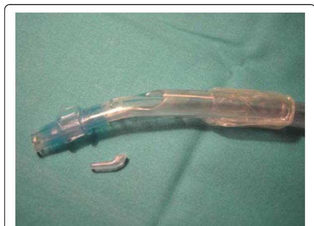
**Figure 1** Amputation of the carinal hook (arrows) in a left-sided polyvinylchloride Carlens DLT (SUMI<sup>®</sup>, Portex Inc., Mexico).
