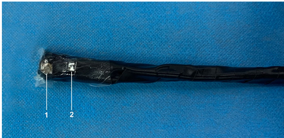
Fig. 1 The modified transesophageal oximetry sensor. 1 detector of the oximetry sensor, 2 emitter of the oximetry sensor
